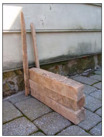
Photo 4. Some of the components of the wall infill. Mud and grass was packed around each of the horizontals which spanned between the bent posts of the house.
