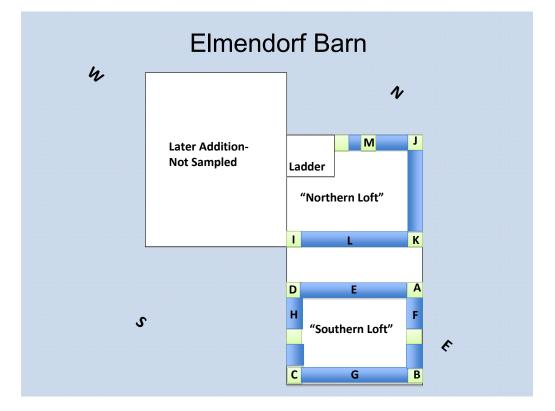
Figure 1: Plan of the Elmendorf Barn with sample posts and beams labeled by letter. Posts and a stud are represented by yellow squares and beams by blue rectangles.
