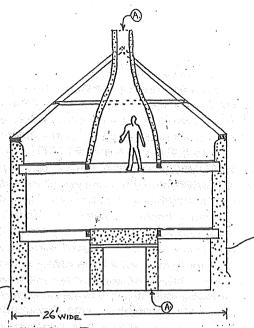
Section B. The later jambed fireplace below the jambless on the west end-wall has been elliminated in these drawings. See page 8. for an explination of the figure in the smoke hood.
